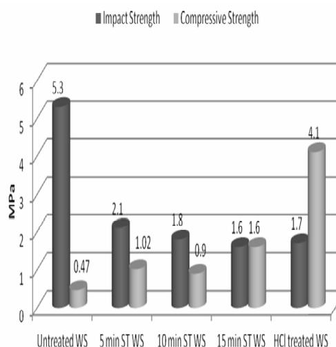
Fig. 2: Effect of wheat straw pretreatment on Impact Strength and Compressive Strength of experimental pellets of Particle Board.
