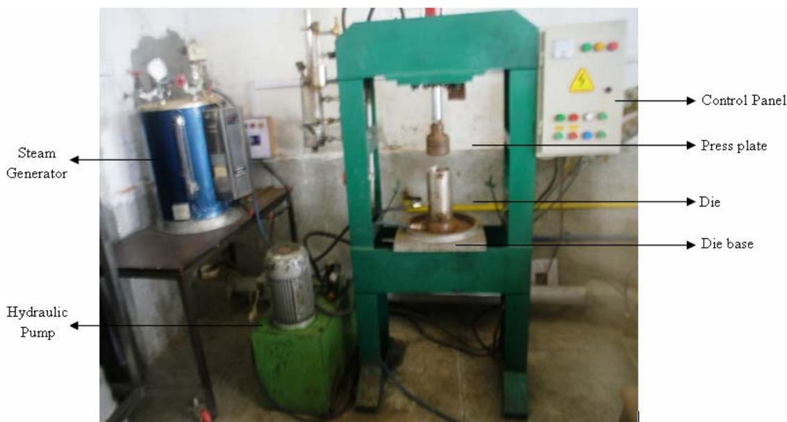
Fig. 7: Mechanical Thermal Compression Rig.
