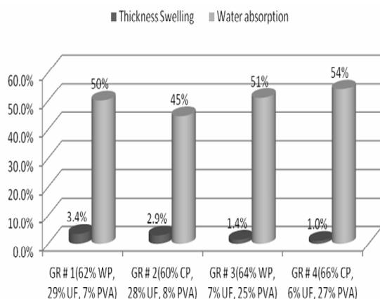
Fig. 6: Effect of glue recipes on Thickness Swelling and Water Absorption of experimental pellets of Particle Board.
