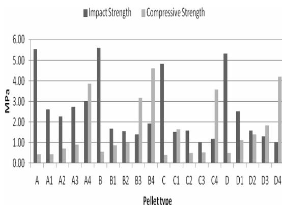
Fig. 1: Compressive Strength and Impact Strength of experimental pellets of Particle Board
