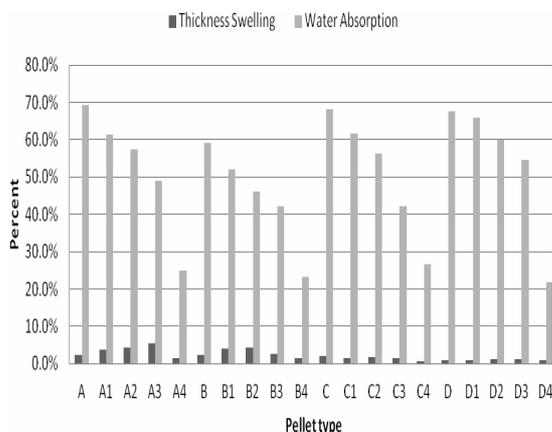
Fig. 4: Thickness Swelling and Water Absorption of experimental pellets of Particle Board.
