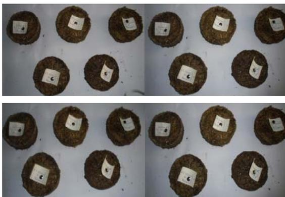
Fig. 8: Particle Board Pellets produced with different feed conditions and glue recipe
