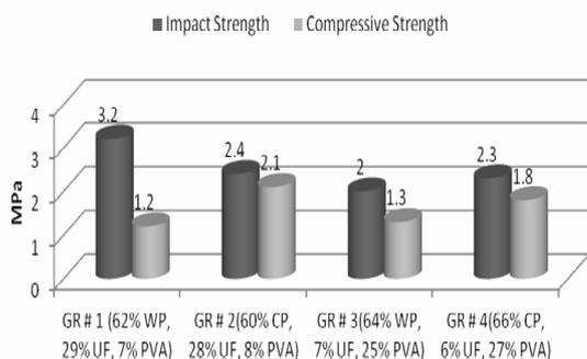
Fig. 3: Effect of glue recipes on Impact Strength and Compressive Strength of experimental pellets of Particle Board.
