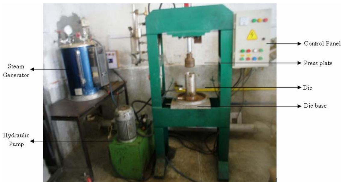
Fig. 7: Mechanical Thermal Compression Rig.
