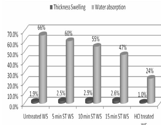
Fig. 5: Effect of Wheat Straw pretreatment on Thickness Swelling and Water Absorption of experimental pellets of Particle Board.
